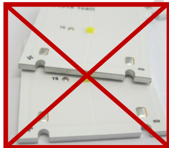
Figure 3c. Incorrect handling of WICOP LEDs
